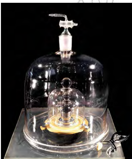
Figure 3.42 The international prototype kilogram has a mass of exactly one kilogram.
