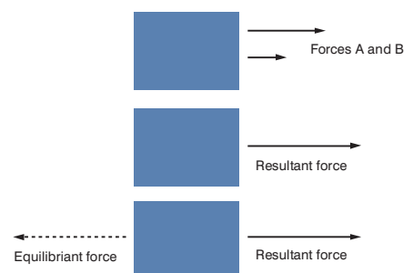
Figure 3.29 There are several forces acting on an aircraft in flight.
